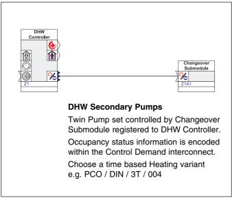
The Changeover Submodule will operate the pump set continuously during the Occupancy Times of the parent module, including Optimum Start and Stop.
