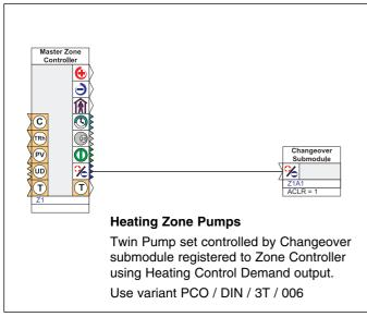
The Changeover Submodule will operate the pump set only when there is a Heating Demand > 5% from the Zone Controller.
