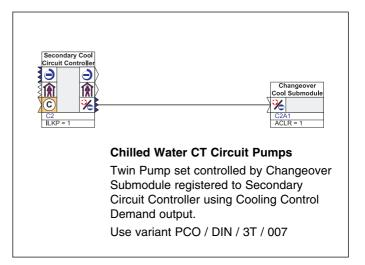
The Changeover Submodule will operate the pump set only when there is a Cooling Demand > 5% from the Secondary Circuit Controller.
