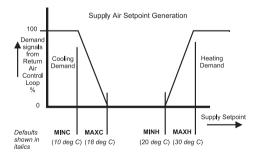
With no Sensor fitted, the Fan Coil Controller will adjust its heating and cooling outputs to the valves etc. on the basis of the demand signals received from the Zone Controller or "Master" Fan Coil Controller (e.g. if the Zone Controller is demanding 50% Heat, the heating valve will be driven to 50% open). This is called *Open-Loop Control* ).
