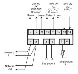
IMPORTANT All network and input cables from flowswitches or contactor status signals to be unscreened, twisted pair cable 20AWG
