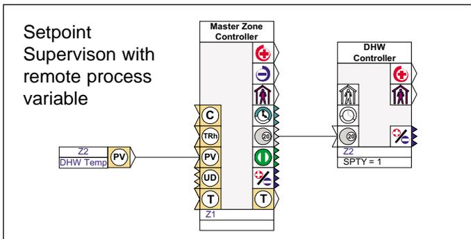
Zone Controller displays (and uses) the DHW temperature as its process variable in place of the room temperature.
