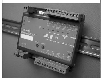
If multiple demands are being received from other modules requiring Primary CT water (for instance, another VT circuit controlled by a Secondary Circuit Controller, or a Domestic Hot Water load) the Boiler Primary Control Temperature setpoint will automatically be raised to the correct value to satisfy the Module with the highest demand. Modules that require Primary (CT) water send their Demand signals in the form of a setpoint, which is high enough to account for Primary losses.
